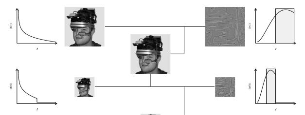
Top: Spatial foveation [1]. First, a Gaussian multiresolution pyramid is created for each input frame (left). For each pixel in the output image (right), a cutoff frequency is specified in retinal coordinates. Pixels are either taken directly from a pyramid level (along the circles) or interpolated between two adjacent levels. Here, an exponential falloff of resolution towards the periphery is simulated, but arbitrary resolution maps can be defined.
