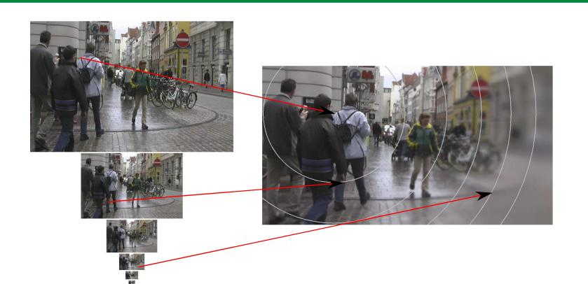
Foveation approaches based on Gaussian pyramids (see left) only allow to specify a cut-off frequency per pixel in retinal coordinates. We now extended our algorithm to be based on a spatio-temporal Laplacian pyramid, which allows to assign a set of (gazecontingent) weights to individual frequency bands.
