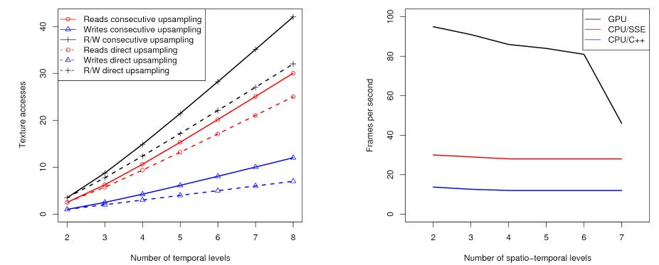
Left: Instead of iteratively upsampling temporal levels as in [2], we use 'direct upsampling' for a performance gain of about 20%.
